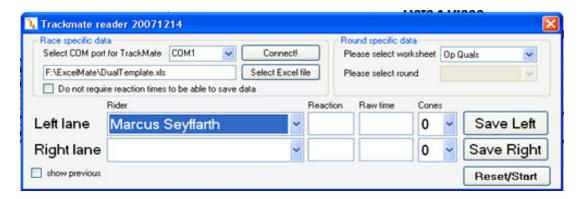
Select the COM port that you connected the cable to (or the one you have assigned your USB converter to act as during installation of your USB to RS232 converter cable). All available COM ports on the computer should be in the dropdown list and selectable.
